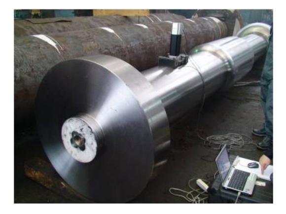
The test subject was forged shaft that was tested by applying curvature magnet system. Purpose of the test was to evaluate change of properties per each processing stage and change of residual stress.
