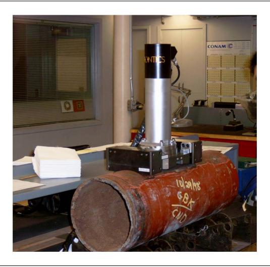
The test subject was natural gas pipeline, to which curvature magnet system was applied, considering the shape. Purpose of the test was to compare between the properties of the materials used for over a couple of decades and that of the new material.
