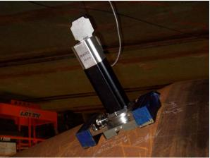
Curvature magnet system - Dovetail Slider
